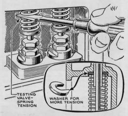
Washer Quiets Knock. A knock may occur at idling speed if the camshaft gear is worn and one or more valve springs do not have sufficient tension. W. M. Dierks, of Chicago, says such knocking usually can be quieted in the following way. With the engine idling, insert a screwdriver into each spring. When the knock stops, you've found the faulty one. Force a horse-shoe washer 1/16" thick under the seat.
