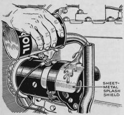
Shield Protects Generator. While filling up with oil, you may have noticed that the attendant sometimes allows a little to slop over the filler tube. Ray Wolfram, of Chicago, writes that he finally traced a mysterious generator trouble to such carelessness. Spilled over the generator, the oil had fouled the brushes. To prevent this from happening again, he installed a metal shield as shown.
