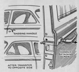
Reverse Sagging Handles. On some cars the door handles eventually wear enough so that they sag below the chrome strip they were designed to parallel. Don E. Braman, of Little Rock, Ark., found a simple solution for this on his 1941 Chevrolet. Removing the handles, he transferred each to the door on the opposite side. There, since the worn part was up, the handle didn't sag. Three minutes did the job.
