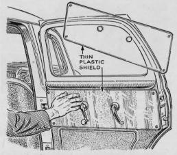
Plastic Keeps Door Clean. Most everyone these days installs seat covers in a new car, but few give any thought to the door areas, where hands frequently soil the covering material. Frank J. Montemuro, of Philadelphia, is one person who does. Cutting a sheet of clear plastic to fit, he installed it as a shield around the door and window handles on each door. The plastic is easily wiped clean.
