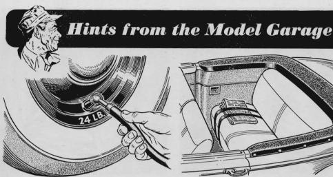
Prevent Overinflation. The new low-pressure tires are sometimes overinflated through carelessness. As a reminder to service-station attendants, paint the correct pressure on the rim beside each valve stem with white enamel, or apply waterproof adhesive tape with the figure inked on. You can also buy markers for your caps. See page 169.
