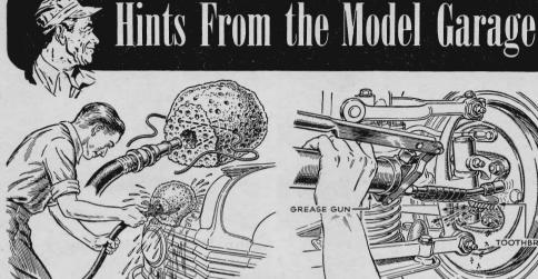
Washing Job Speeded Up. You can do a better job of washing a car if a sponge is attached to the nozzle of the hose. Cut a blind hole just large enough for insertion of the nozzle. Run heavy cord through with a needle and tie to the hose.
