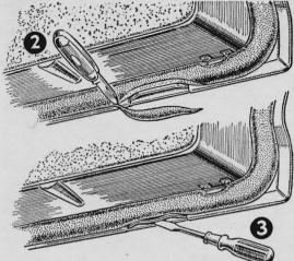
**Drain Slots Need Cleaning.** You should check over the drain slots in the door and body panels of your car occasionally. Otherwise, pent-up water may rust the metal.
