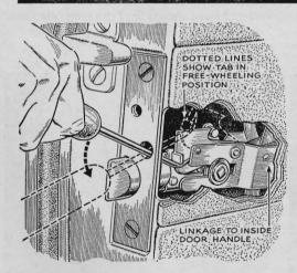
Keep Children Safe. Did you know there's a safety feature in the rear doors of General Motors four-door sedans? With a pointed tool (for instance, an ice pick with the point slightly bent), you can adjust the lock so the inside handle won't open the door. The handle is as easily returned to operation. GM introduced these locks in 1941. They've been used ever since in all models except '46, '47, and '48 Buicks.
