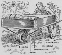
Trailer Used as Wheelbarrow. It's difficult to handle a caster-type trailer when detached from the car. F. W. Sewell, of San Mateo, Calif., overcame this by rigging his like a wheelbarrow. A ringbolt was attached to the body at each side. When the trailer is to be moved, removable chains with S-hooks in each end keep the wheel rigid. Turnbuckles tighten the chains. A sawhorse supports the trailer.
