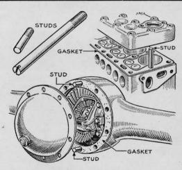
**Special Studs Align Parts.** In the garage where A. G. Patrick works in Hot Springs, Ark., you'll find a small box containing bolts of various sizes. These are not ordinary bolts, however. The head has been removed from each, and slots have been cut in some. As illustrated, these are often useful for keeping parts aligned during assembly. With several screws in, studs are removed with pliers or a screwdriver.
