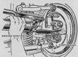
Brush Off the Fitting. An old toothbrush with stiff bristles is ideal for cleaning grease and embedded dirt from grease fittings before applying the gun. For greater working convenience, tape the handle of the brush to the nozzle of the gun.
