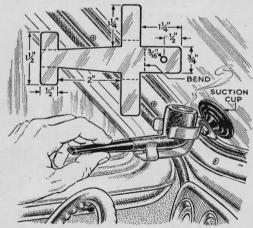
Clip Supports Your Pipe. If you smoke a pipe while driving, you can give your jaws a rest occasionally with this clip. Copper or aluminum is easiest to work, but brass is more springy and makes a better clip. Using the pipe as a guide, bend the metal to shape. A suction cup with a screw molded into it can usually be found in an auto store. The clip was designed by Arthur Trauffer, of Council Bluffs, Iowa.
