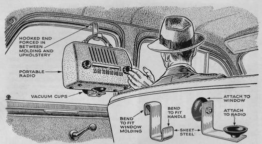
**Portable Used in Car.** Installed as shown, a good portable can double as a car radio. You'll notice that it can be quickly dismounted to serve in its original function.
