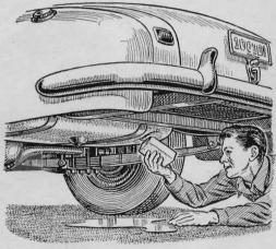
**Soap Stops Gas Leak.** If carefully applied, a bar of soap will make an emergency roadside repair for a small leak in your gas tank. After locating the hole, wipe off surrounding dirt and grease and rub the soap firmly over the spot several times. Since gasoline will not readily dissolve soap, this temporary fix will usually last until you can get to a garage and have the tank repaired or replaced.
