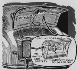
Light Works Automatically. If your luggage compartment hasn't a light, here's one that you can install at little expense. Mount a mercury switch under the lid to close the circuit and turn on the light automatically when you lift the lid. Drop the lid, and it goes off. Tap a taillight wire for the hot lead, and provide a good ground contact from the reflector to the car. A tin can cut in half makes a good reflector.
