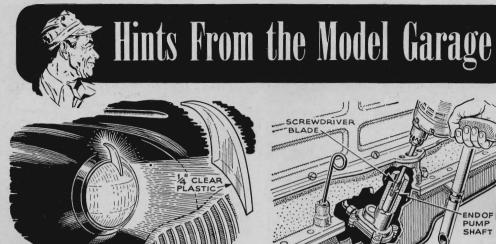
Plastic Shows Lights Are On. If a headlight burns out, you'll know it without leaving the car. Edge-lighted along the lower surface, a horn-shaped indicator cut from plastic carries the illumination up where you can see it. A good cement job will hold it on, or a metal strip screwed to rear corner can be clamped by lamp rim.
