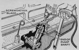
Drill Primes Pump. When an engine is started after an overhaul, oil pressure must come up fast to protect dry, tight wearing surfaces. Reader George Pedley, working on a Chevrolet engine, used an electric drill to run the pump until the oil gauge showed pressure. Then he finished assembly, timed the engine, and started it.
