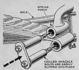
Cold Shackle Goes in Easily. Since cold contracts metal and hardens rubber, Robert Douglas, of Rochester, N. Y., suggests that you take advantage of this when installing Ford or similar spring shackles. Put the new ones into the freezing compartment of a refrigerator and leave for about half an hour. Then you'll find they have contracted enough to go into place with much less difficulty.
