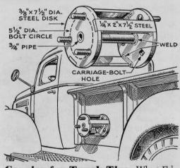
Carrier for Truck Tire. When Edward S. Barrows, of Philadelphia, bought a pickup, the spare-tire carrier was missing. He remedied this by building the one illustrated from scrap materials. He writes that he finds this more convenient than the usual carrier under the box and that it doesn't interfere with any use of the truck. Should you want to carry an extra spare, a carrier like this might be the answer.
