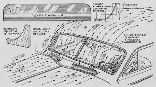
Bugs Kept Off Windshield. At this season, the spatter and smear of insects on a windshield makes seeing tough, especially at night. A. W. Schach, of Rockford, Ill., uses deflectors like these to overcome the problem. The sketch on ½" squares
