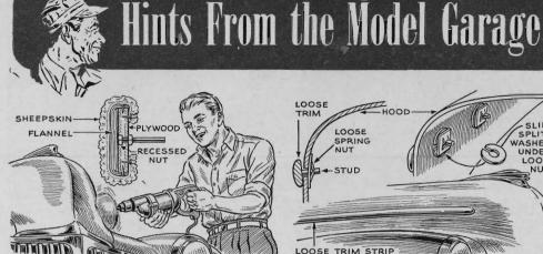
Make Your Own Polishing Pad. If you own an electric drill, it's a simple job to assemble a polishing attachment. Cut a 5" disk from 1/2" plywood, drill and counterbore it, and attach a shaft cut from a 4" bolt. Pad the face with several layers of flannel. Finish it off with sheepskin cut from a polishing mitt, tacking along the back.
