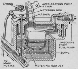
Carburetor Service Tip. In a modern carburetor of the metering-rod type, the little spring at the top of the metering rod and the sealing washer are points that occasionally give trouble. If the spring is missing, the rod may vibrate sufficiently to unseat the washer. This admits full atmospheric pressure to the chamber. Rough engine performance or high fuel consumption may sometimes be traced to this.
