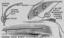
Washers Tighten Trim. Chromium trim often is attached with unthreaded studs and flat spring nuts. In time, wear on the studs may loosen the nuts and allow the trim to rattle and squeak. One way of tightening it is suggested above. Cut a section from a steel washer. Then force the washer behind the nut to take up the slack.
