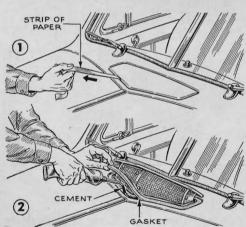
Repairing a Cowl Ventilator. Water may leak through a cowl ventilator unless the lid makes firm and even contact with the gasket. If a strip of paper can be withdrawn when the lid is closed on it (1), increase the lid tension by shortening the adjusting link you'll find under the instrument panel. It's also sometimes helpful to remove the gasket, clean it and its channel, and carefully cement in place (2).
