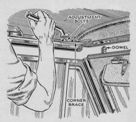
Adjusting a Folding Top. Convertible tops on General Motors cars may be adjusted either forward or back if the dowels don't hit their holes in the roof rail. First, unlatch the top and raise it slightly. Next, loosen the adjustment bolts. Then move the corner brace until the dowels and holes are properly aligned. In some cars, a different corner brace is used, but the adjustment is essentially the same.
