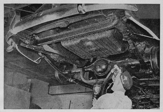
**SPRAY PROTECTS CHASSIS.** A rubberized material developed by the Minnesota Mining & Manufacturing Company, of Saint Paul, Minn., may be sprayed on the underparts of a car as a protective coating against corrosion, moisture, and flying sand or grav-
