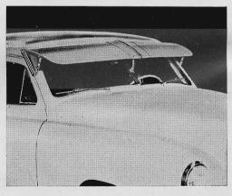
SHADE CUTS SKY GLARE. A sheet-aluminum shade with stainless-steel and chrome-plated brass fittings affords drivers protection against overhead glare. It is made by the Fulton Company, of Milwaukee, in sizes to fit most popular and de luxe models of 1942, 1946, and 1947 cars and many others of older make.
