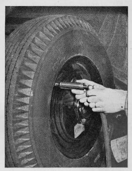
**Powder Suppresses Static.** Powder that is said to overcome the insulation property of rubber tires and prevent static electricity from building up in a moving car will soon come on the market. An air hose and a special container are used to inject a tablespoonful into each tube after the valve core has been removed. The United States Rubber Company developed the powder as an outgrowth of research on conductive tires for vehicles in industrial plants where a spark would be dangerous.
