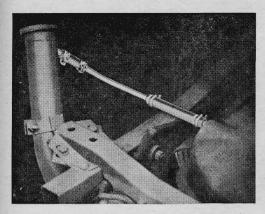
PREVENTION OF GAS LOSS through spilling and evaporation when the tank is being filled is the object of an air-pressure relief pipe leading from the tank to the filler pipe on the new 1947 Studebakers. The relief pipe releases air that would otherwise cause the gasoline to foam and gurgle as the level rises in the tank. It was designed after a study of waste from this cause.
