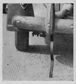
A RUBBER GROUND strip for carrying off static electricity from fuel and other trucks has been developed by the U.S. Rubber Co. Made of a special conductive rubber, the strip grounds the frame so any static electricity can pass off harmlessly. Besides being noiseless, the rubber is said to wear longer than the conventional chain.
