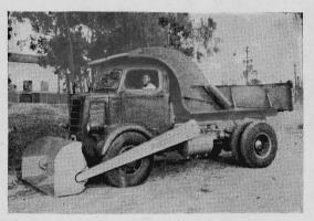
With shovel lowered, the truck above moves forward to scoop up a load of earth. Then, swinging the load up and back, the driver dumps it, below, into the truck.
