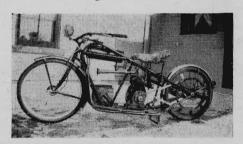
BICYCLE WHEELS mounted on a frame of thin-wall conduit and powered by a  $2\frac{1}{2}$ -hp. motorcycle engine form the basis of this motor bike built by Edward Stuebe, of Watertown, Wis. The machine can do 35 miles per hour.
