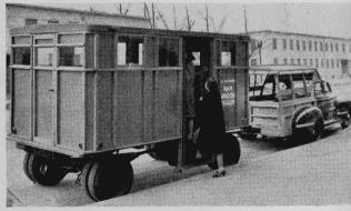
LIGHT TIRES ON THIS TRAILER and wood instead of steel construction save critical materials in the transportation of war-plant and other workers. The trailer mounts eight tires of the new Victory type that use but a few ounces of crude rubber compared to the 60 percent of crude required for heavy bus tires. The trailer seats 24 persons, and the converted sedan pulling it carries 15 more.
