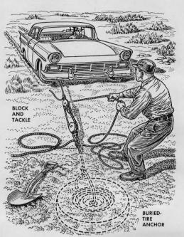
Block and tackle won't pull your car out of a soft back road or a sandy seashore if there's no place to secure the ropes. An effective "deadman" can be made by burying the spare wheel—the deeper the better—and using it as an anchor.
