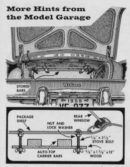
A car-top carrier can be neatly stored in the unused space beneath the rear package shelf in a sedan. Lock four long bolts in the shelf so they protrude into the trunk. Use wing nuts and wood strips to clamp the carrier between the bolts.
