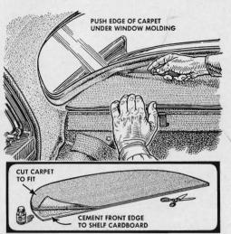
You can silence the rattling of loose objects on the package shelf by fitting it with carpeting. Appearance will be improved, too. Cement the front edge of the carpeting to the shelf, and tuck the other edges under the rear-window molding.
