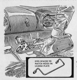
A wire handle on the rear license-plate bracket will end the annoying slamming each time you buy gas. It'll save the rubber bumpers, too, as slamming often causes them to drop off. Bend the handle from heavy wire or a length of brazing rod.
