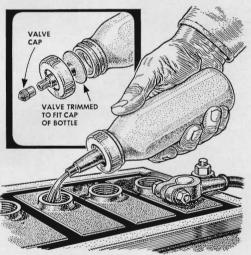
Feed a thirsty battery the exact amount of water it needs without splashing by using a plastic nursing bottle. The rubber nipple can be used by snipping off its tip, or a tire valve can be trimmed to fit, and stoppered with a valve cap as shown.
