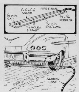
Roads salted in winter? This under-car spray rig will flush away salt deposits as you slowly drive the car into the garage. Place the rig across the driveway and connect it to the garden hose. Drain the hose after using so it doesn't freeze.
