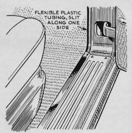
**Frayed door piping** can be improved in appearance, or the piping in a new car protected, by covering it with flexible clear-plastic tubing. Slit the tubing along one side and force it over the piping. Tuck the ends under the metal step plates.
