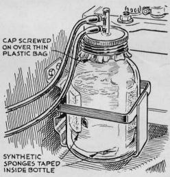
**Fool old man winter** by placing several synthetic sponges and a plastic bag inside the windshield-washer bottle. Fill the bag with water and solvent. If the solution should freeze, the sponges and bag will allow for expansion.
