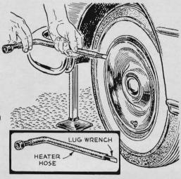
**Protect your hands** from contact with chilled metal by slipping a length of heater hose over the shank of your lug wrench. The hose will also keep the wrench from marring rims or whitewalls when prying off wheel covers.
