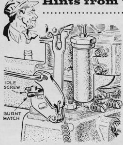
To increase idling speed temporarily when you charge the battery with the generator, or warm the engine, insert a burnt match between the carburetor idle screw and its stop. When you step on the throttle, the match will drop away.
