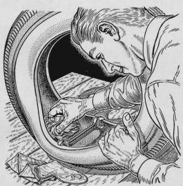
You can quickly locate a nail or a sliver of metal inside a tire casing by wiping the casing with a discarded silk or nylon stocking. The filmy fabric will snag on the tiniest irregularity in the normally smooth rubber, signaling its location.
