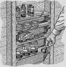
For out-of-the-way storage of cans and small parts in the garage, bridge the empty spaces between wall studs with a number of 1" shelves about 3\%" wide. Cleats can be nailed to the sides of the studs to support the shelves.
