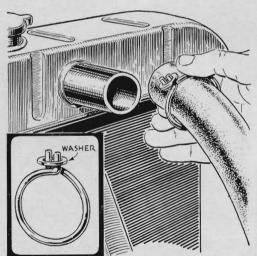
**Installing a wire hose clamp** in tight quarters needn't be a knuckle-buster. Before slipping the clamp on the hose, expand it until the ends touch and slip a small washer over them. When the hose is in place, pull off the washer.
