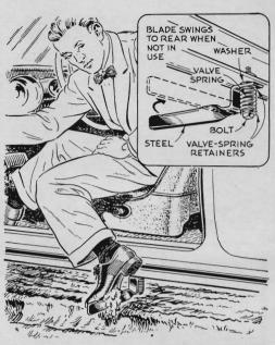
With a shoe scraper always handy, mud and slush needn't dirty up the inside of a car. This swing-in, swing-out blade bolts to the car frame, and because it's springloaded stays put except when pushed sideways by the user's foot.
