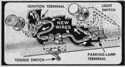
Wiring parking lights separately through the ignition switch automatically turns them off when you cut the engine after the early-morning trip to the station. A toggle switch permits use of parking lights with headlights for special effect.
