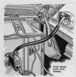
A hard-to-reach master cylinder can be filled with brake fluid through a short length of hose and a funnel. Insert the hose in the cylinder opening and slowly pour fluid into the funnel. Check the level occasionally to avoid overfilling.
