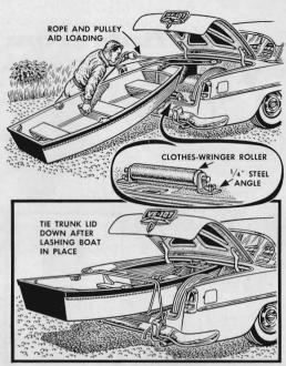
You can load a pram single-handed in the trunk of your car with this setup of pulley and wringer roller. Rest the bow on the roller, and ease the weight off the stern as you pull the pram into the trunk with the rope and pulley.
