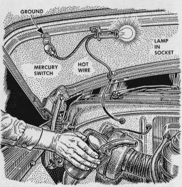
An automatic light that turns itself on when the hood is raised is a convenience when servicing your engine at night. A tail-light bulb, socket with bracket and mercury switch can be purchased at any auto-supply store. Connect as shown.
