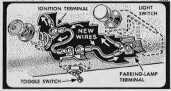
Wiring parking lights separately through the ignition switch automatically turns them off when you cut the engine after the early-morning trip to the station. A toggle switch permits use of parking lights with headlights for special effect.
