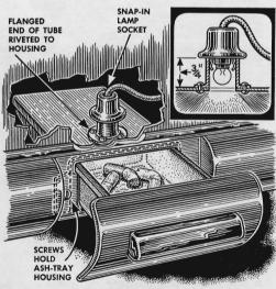
Find your ash tray in the dark by adding a light to its housing. Unscrew the housing, drill a hole in its top, and rivet or solder a short length of 1/2" tubing over the hole. Install a snap-in socket and run the wire to the dash-light switch.
