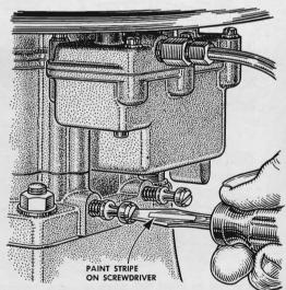
It's easier to count the turns when adjusting the idle screws on a carburetor if you paint a mark on one side of the screwdriver blade. Each time the mark comes into view, you know you've made one complete turn; no mark, a half turn.
