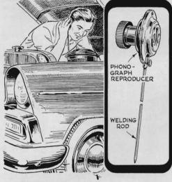
**Faint bearing knocks** can be detected by the mechanical reproducer from an oldstyle or child's phonograph. Fit a length of thin welding rod or coat-hanger wire into the needle holder and slip a makeshift rubber earpiece over the sound tube.
