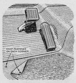
**Anchor floor mats** that shift around or curl up at the edges with snap fasteners. You can find suitable sew-on or hammerin fasteners at the sewing counter of any five-and-ten or notions store. Attach one at each corner of the floor mat.
