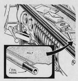
A felt dash cover prevents sunny reflections on a bright day and creates non-skid storage space for small articles. Sew the cover's rear edge around some hose; this forms a rim to keep the items on top of the dash from falling off.
