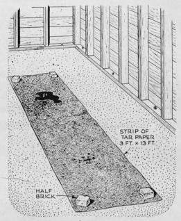
**Grease and oil drips** won't dirty a garage floor if you put down a strip of asphalt building paper. The oil catcher is held down by half-bricks that can be moved easily when you want to replace the strip or clean the garage.
