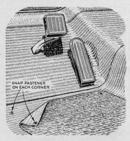
Anchor floor mats that shift around or curl up at the edges with snap fasteners. You can find suitable sew-on or hammerin fasteners at the sewing counter of any five-and-ten or notions store. Attach one at each corner of the floor mat.
