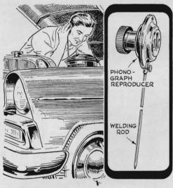
**Faint bearing knocks** can be detected by the mechanical reproducer from an oldstyle or child's phonograph. Fit a length of thin welding rod or coat-hanger wire into the needle holder and slip a makeshift rubber earpiece over the sound tube.
