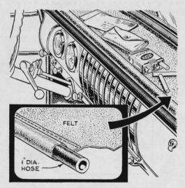
A felt dash cover prevents sunny reflections on a bright day and creates non-skid storage space for small articles. Sew the cover's rear edge around some hose; this forms a rim to keep the items on top of the dash from falling off.
