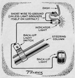
When your car is in reverse, this light blinks on to warn you. It's bracketed to the underside of the dash and wired to the back-up light switch. When the backup lights go on, so does the dash light as a visual reminder to the driver.
