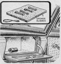
Spare fuses and bulbs won't get smashed by tools, flashlights and such in your glove compartment if they're protected by foam rubber. Roll them up in a small sheet of the resilient material and wrap this with a heavy rubber band or two.
