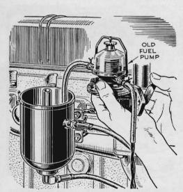
Cleaning out the oil-filter housing during an oil change is messy when the housing has no drain plug. For this difficult job I use an old, but workable, fuel pump. Moving the actuating lever by hand sucks out the sludge in the bottom.
