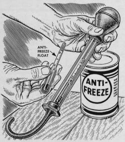
A hydrometer can do double duty if you buy a second float calibrated for antifreeze. Remove the tip of the tester to install the proper float for checking the battery or the antifreeze. Rinse the hydrometer with clear water after each use.
