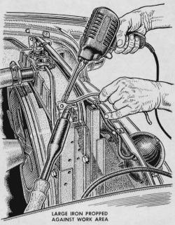
Concentrate extra heat into an area that's difficult to solder by propping the tip of a large iron against the spot while you do the actual soldering with a second iron or a gun. Drain out the coolant when working on a radiator or heater.
