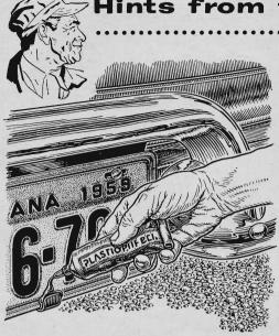
Rattles can be silenced where metal vibrates against metal, as often with license plates, by flowing a bit of liquid rubber between the offending parts. The rubber can be molded into an invisible cushion that remains soft after it dries.
