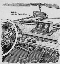
**Extra meters** can be installed without cutting the dash. House them in a radio utility box on top—where the speaker grille is often found. If you want to remove them, the grille can be cheaply replaced, leaving no holes in the dash.
