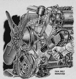
Take the hazard out of timing the ignition by removing the fan belt before tuning up. The engine will idle the same without it, and you can safely reach down with the timing light to pinpoint the degree marks on the vibration damper.
