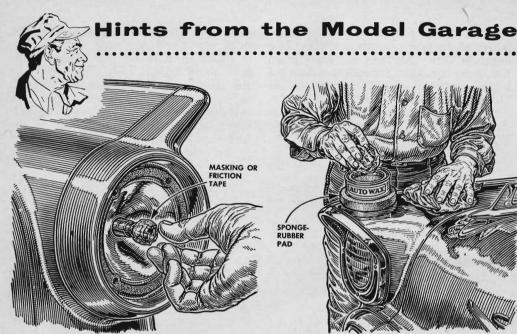
To remove a frozen light bulb-one stuck in the socket by corrosion-wrap the glass with masking tape. This will provide a non-slip grip and protect fingers from fragments of glass if the bulb should break when forced inward and twisted.
