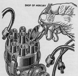
A perfect connection can be made between high-tension spark-plug wires and the terminals of the distributor cap by putting a drop of mercury in each terminal. The mercury closes the gap between wire and contact, preventing corrosion.
