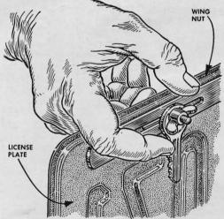
Hiding an extra ignition key behind the license plate may save you a broken vent window if you should inadvertently lock your key inside the car, or misplace it. Enlarge the hole in the key to 1/4" and secure it with the license-plate bolt.
