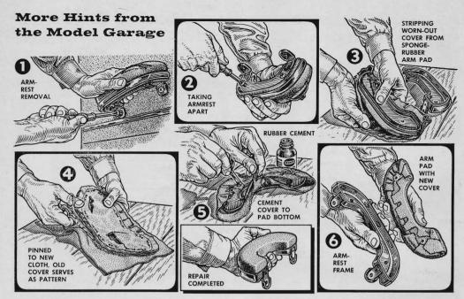
**Armrest repair.** As a car grows older it's natural that the armrest on the driver's door should wear through on the top. When this happens, a new cover can be put on easily, using material that either matches or contrasts with the original up-
