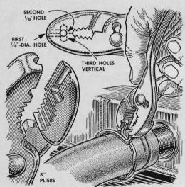
Make a handy hose-clamp tool from inexpensive slip-joint pliers by drilling three ½" holes. Clamp the jaws and drill one hole from the end, another in from one side. Open the jaws and drill each where the first two holes intersect.
