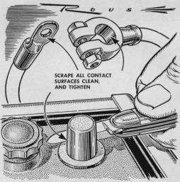
When lights burn out mysteriously, check for loose battery connections or a corroded ground strap. (An intermittent bad connection can result in generator-caused overvoltage.) Scrape all surfaces bright, and tighten for good contact.
