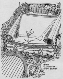
Where maneuvering is tight or the beach very shallow, try hooking your boat trailer to a hitch clamped to the front bumper. With this setup, you can quickly correct the trailer if it drifts off course, and push it right to the water's edge.
