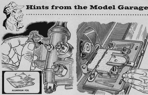
Grease fittings can be kept clean between lube jobs by pressing little squares of household aluminum foil over them. Covering the fittings takes no longer than wiping them clean, and eliminates the danger of forcing grit into the bearings.
