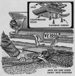
A sled-like base of heavy sheet metal fastened to the bottom of a jack will keep it from tipping and help it slide easily as it is pushed under the car over gravel or loose earth. The base also minimizes sinking into soft earth.
