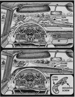
You can shield your eyes from hood glare, when driving toward the sun, by placing a strip of cardboard across the bottom of the windshield. Cut the strip to block out the hood—not the road—and screw metal clips to the molding to hold it.
