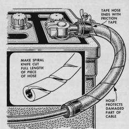
Reinforce heavy insulation, or cover it if it's frayed, by wrapping with garden hose. Use a sharp knife to cut a continuous spiral from a piece of the required length, then wrap it around the wire. Twist it tight and tape the ends.
