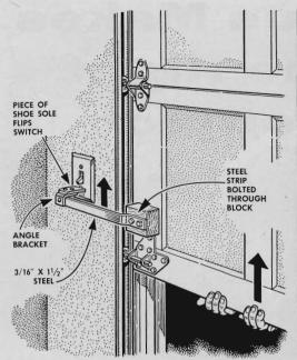
Automatic garage-light switch is actuated by a leather "thumb" mounted on an extension arm on the garage door. The leather tab must be stiff enough to flip the toggle as the door is raised or lowered, yet flexible enough to brush past it.
