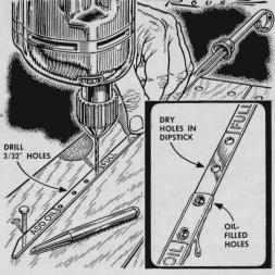
Reading the crankcase dipstick will be easier, especially when the oil is fresh and clear, if you drill four small holes between the FULL and ADD OIL marks. The holes covered by oil will appear as tiny lenses; the others will remain open.
