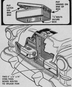
**Extra storage space** for tools, oil, flashlight and spare parts can be obtained by bolting a steel tool box behind the grille on each side of the radiator. Be sure to locate the boxes so they can be reached easily and do not obstruct the radiator.
