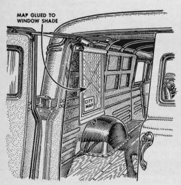
A large map that is referred to frequently can be made instantly available by pasting it to a window shade. Use flexible cement or photo-mounting tissue. Hang the roller on shade brackets in a place where it can easily be pulled down.
