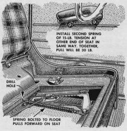
Adjusting the front seat is easier for a short person if a pair of screen-door springs are attached to pull it forward when the lock is released. A tall driver can readily overcome the spring tension and push the seat back again.
