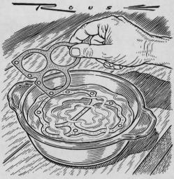
When re-using gaskets after minor carburetor repairs, soak them in water or kerosene while you work on the assembly. The fluid causes the gaskets to expand and their fibers to fluff up to full thickness. Treat new gaskets the same way.
