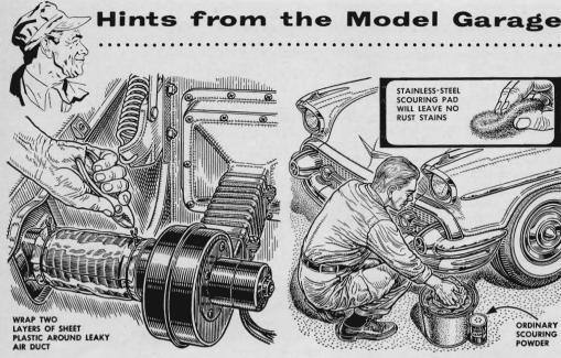
Seal out engine fumes—if they're finding their way into your car through pinholes in the heater duct—with a simple but effective boot of plastic material. Wrap the material twice around the duct and close the ends with wire, twisted tight.
