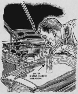
A glass of water placed on the front fender will guide you when adjusting the carburetor. Turn the idling screws in or out until the water is least agitated. At this point, the jets will be set for the smoothest idle possible.
