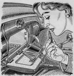
A dash vanity like this will make a hit with lady passengers. Solder hinges to the metal back of a small mirror and mount it inside the glove-compartment door. The compartment light will illuminate the area for face fixes at night.
