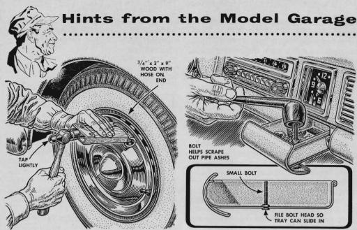
Wheel covers can be driven securely in place without denting them with this quickly made tool. Round off one end of a piece of wood and cushion it with a short length of heater hose. Fasten a steel plate around the hammering end.
