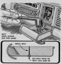
A pipe reamer, made by locking a 1" or 11/2" machine screw in a hole drilled in the bottom of the ash receptacle, will clean out the bowl neatly. Countersink the screw head or file it nearly flush if it catches when the tray is pushed in.
