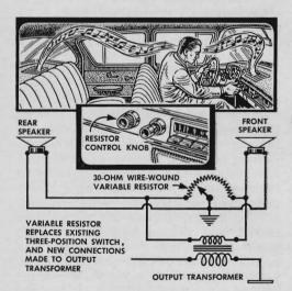
Volume of front and rear speakers can be delicately adjusted with a variable resistor. Centered, the control puts both speakers at equal output. Turned to either side, it gradually reduces the volume of one and steps up the other.
