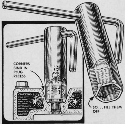
A spark-plug wrench will work easier if you file off the sharp outside corners. This small effort will prevent the six-sided wrench from binding or digging into the plug-recess sides as you exert pressure to loosen or tighten the plug.
