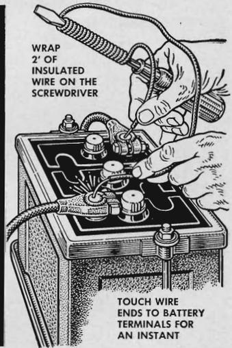
If a nut or bolt drops into an out-of-reach place, retrieve it with a magnetized screwdriver. Wrap the tool with insulated wire and briefly touch the ends to the battery. Then tie the wire to the handle and lower it to pick up the part.
