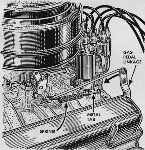
**Erratic idling**—fast one time, slow the next—can often be corrected by adding a 10-cent spring to the throttle linkage. Stretch the spring far enough to insure positive throttle return, and secure it to a metal tab held by a head bolt.
