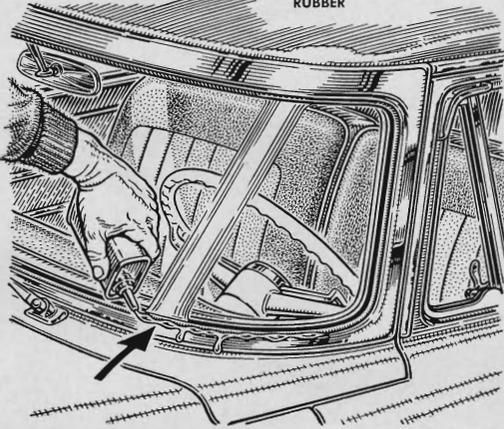
To stop an annoying squeak caused by vibration of the windshield in its opening, trickle silicone rubber lubricant between the metal molding and the rubber channel. If this doesn't silence it, force sealing compound between rubber and glass.
