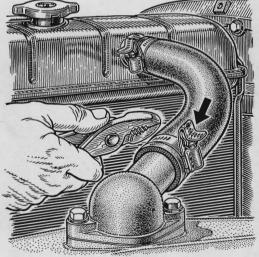
Tighten a hose clamp with this neat trick, copied from the Air Force system of securing bolt heads with wire: Bend the end of a gear-band hose clamp over the thumbscrew after it's been tightened. Now vibration can't loosen the clamp.
