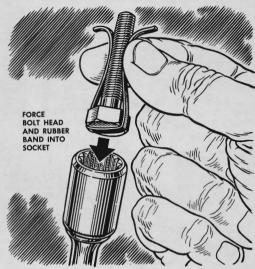
To start a bolt in tight quarters try holding it in an extension socket with a piece of rubber band. Stretch the rubber over the head of the bolt and force it in the socket. When the bolt is seated, the socket can be easily pulled away.
