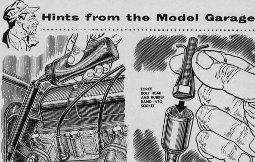
Plastic squeeze bottles make short work of adding lubricant or fluid at hard-toreach places on a car. Slice a little off each spout to enlarge the hole, and fill bottles with the proper oil for transmission, brake cylinder and differential.
