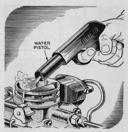
To start a balky engine or save cranking to prime the fuel system after running out of gas, fill a metal water pistol with gas and squirt it into the carb's throat. This is better than *pouring* in gas; the gun breaks it up into a fine spray.
