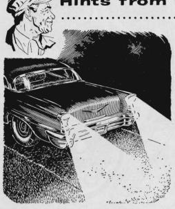
Those big, modern stop lights are brilliant enough to serve as backup lights. To make them go on, touch your brake lightly when backing, or connect them to a separate backup-light switch mounted on the lower end of the steering column.
