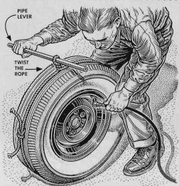
Repair your own tubeless tires? You can seat the beads against the wheel rim so they'll hold air by applying a rope tourniquet around the tire. When partial inflation expands the tire, remove the rope and inflate to recommended pressure.
