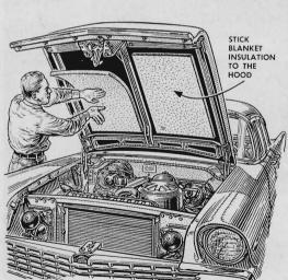
Make your own hood liner from blankettype glass-fiber insulation sold by the yard at lumber yards. Cut the insulation to fit the underside of the hood, apply body undercoating to the metal, and immediately press the material in place.
