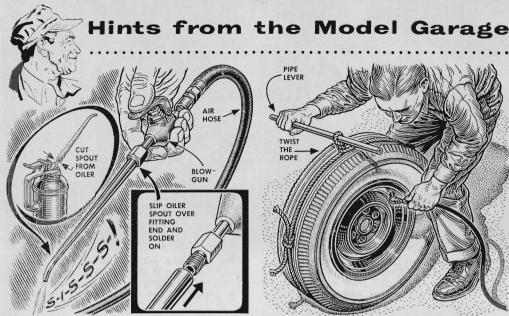
For blowing out dust from inaccessible places, solder the spout from an old oil can to a brass coupling that fits the blowgun nozzle. You can then use the gun for normal cleaning operations and quickly attach the spout for a long reach.
