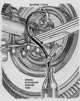
When bleeding brakes with no one to help, a spring clothespin on the bleeder hose serves as a one-way valve to prevent the hose from drawing in air bubbles when the brake pedal is released. Check the master cylinder after bleeding each wheel.
