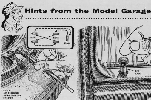
After switching tires, remember to check pressure in the new position. Front tires should carry a few more pounds than rear, and rotating puts the softer rear tires up front (see rotation chart above) where they may prove to be underinflated.
