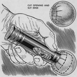
Cap the lens of a flashlight with a rubber ball to protect it while being carried in the trunk, glove compartment or tool box. Cut an opening in the ball, then slit the edge of the opening so it can easily be forced over the lens of the flashlight.
