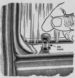
Checking door-lock buttons to see that they're down can be done with a glance if you put a band of red paint or colored tape on them. When the buttons are pressed down, the bands disappear. If you can see a band, the door is unlocked.
