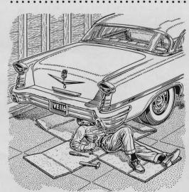
A good makeshift creeper for work beneath your car can be had from a large carton opened flat. It can be shifted about easier than papers or a cloth and the thick board gives your back protection from damp or greasy ground or concrete.
