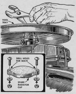
A tip-proof tool tray can be made by bolting a large pie tin or serving tray to the top of a spare radiator cap. Mounted on the radiator's filler neck in place of the regular cap, the tray is handy as you work in the engine compartment.
