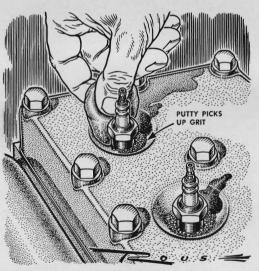
**Pick up dirt and grit** from spark-plug wells, so plugs can be removed without contaminating the cylinders, with a ball of putty or wallpaper cleaner. Press it in firmly, close to the plug. When you lift it out, the grit will adhere to it.
