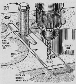
To drill out a broken bolt without damaging the threaded hole, clamp a simple jig under an adjacent bolt to center the drill. To make the jig, cut a slot in one end of a steel strip and drill a guide hole near the other end for the drill bit.
