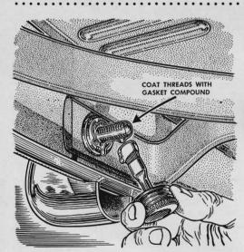
A coating of gasket compound over the protruding end of a bolt exposed to the weather will keep it rust-free and easy to remove. Protect license-plate bolts this way, and coat bumper-bracket bolts, fender and body bolts when new.
