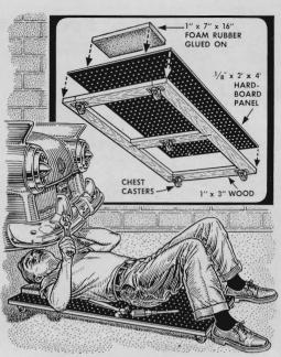
You can build this creeper for about \$4.50, and the investment in comfort will soon be repaid when working under your car. For the frame, join one-by-threes with corrugated fasteners. Cover with perforated hardboard and add casters.
