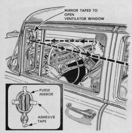
If rearward vision is blocked when hauling furniture or bulky packages, a small hand mirror taped to the outer edge of the vent window on the driver's side will enable you to see. Swing the window to bring the mirror into seeing position.
