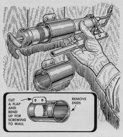
**Storing a grease gun,** calking gun and many other car and home tools is easy in racks made from discarded tin cans. Remove both ends and cut out a flap in the center of the can. Bend the flap outward and screw it to the wall as shown.
