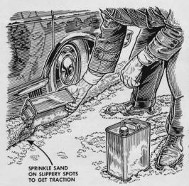
A good way to carry sand for emergency use on ice and snow is in a one-gallon can. Several cans are easy to stow compactly, and sand can't sift through as it sometimes does in bags. Pouring the sand where you need it is easier, too.
